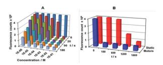
**Fig. 4** Effect of inter-dependent parameters on the quenching of fluorescence intensity of FLA/silica–NH<sub>2</sub>/Pt micromotors: (A) time dependent quenching of micromotors with different concentrations of DCP; and (B) comparison of fluorescent quenching with micromotor and static FLA-coated silica with  $10^{-4}$  M DCP. Reaction conditions: H<sub>2</sub>O<sub>2</sub> (2%), SDS (1%),  $\lambda_{exr}$ , 490 nm;  $\lambda_{emr}$ , 510 nm.
